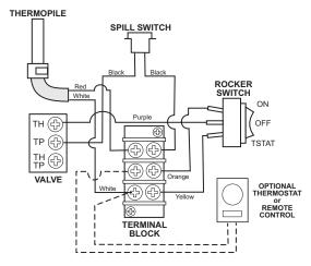
Figure 26. Valve and Accessory wiring diagram.
